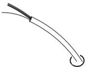
Seal wire hole in wall to prevent cold or hot air from affecting temperature sensor in display
