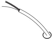
Seal wire hole in wall to prevent cold or hot air from affecting temperature sensor in display.
