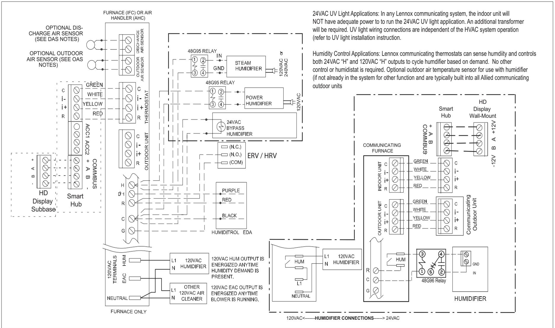
24VAC UV Light Applications: In any Lennox communicating system, the indoor unit will NOT have adequate power to run the 24VAC UV light application. An additional transformer will be required. UV light wiring connections are independent of the HVAC system operation (refer to UV light installation instruction).
