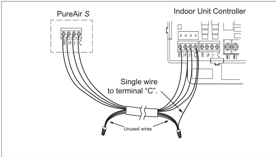
**Figure 12. Communicating Indoor Unit and PureAir S**
